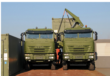
A single Sideloader can load or unload containers from a full convoy of vehicles.
