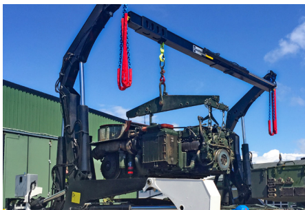
Field service support - here a Sideloader is used to swap the engine of a battle tank.
