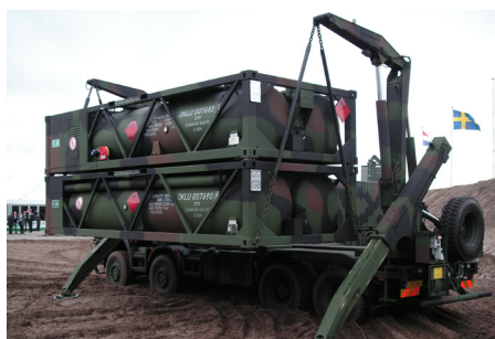
Containerized fuel tanks.
